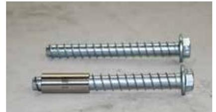
Sleeve can be pushed on completely, screw for No longer suitable for further use
