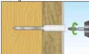
1.1 Screw in the mounting grub screw.
