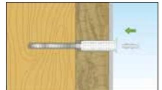
3.1 Drive dowel 5/25 into the decoupling element.
