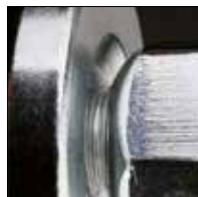
Special washer and rounded nut compensate for small inclinations and unevenness and thus avoid one-sided stress peaks.
